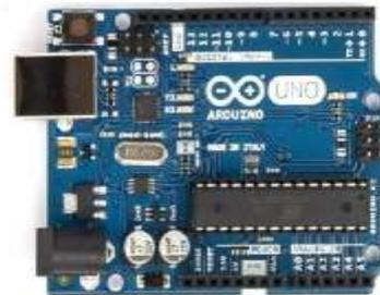
Gambar 1. Board Arduino Uno
